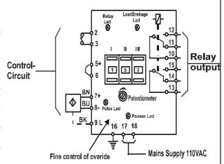
2 & 3 Terminals Relay OK Led 7 & 8 Terminals Pulse Led 17 & 18 Terminals Power ON Led 12,11 & 10 Terminals Lead Breakage Led
